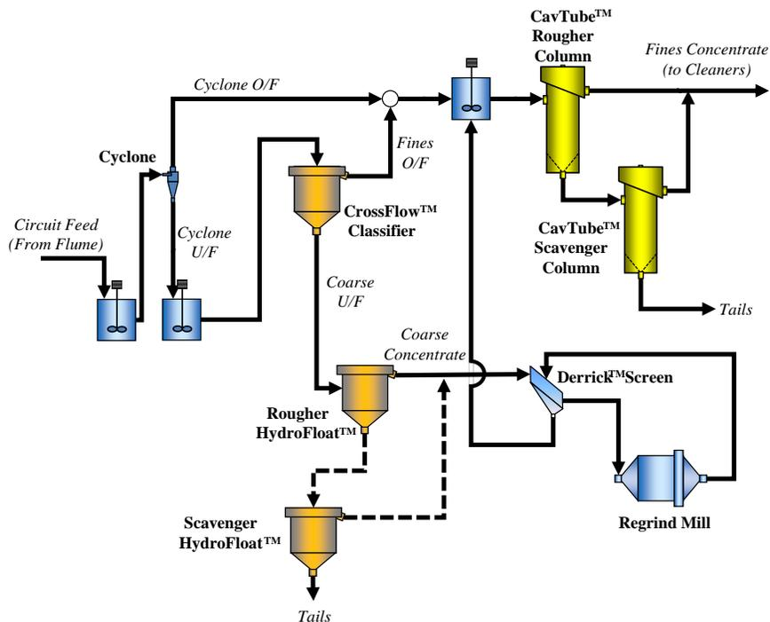
Figure 4 – Schematic diagram of pilot test circuit for copper sulfide tailings treatment
