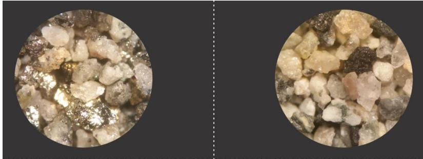
Figure 8 - Microscopic view of +425 concentrate (left) and tailings (right) particles
