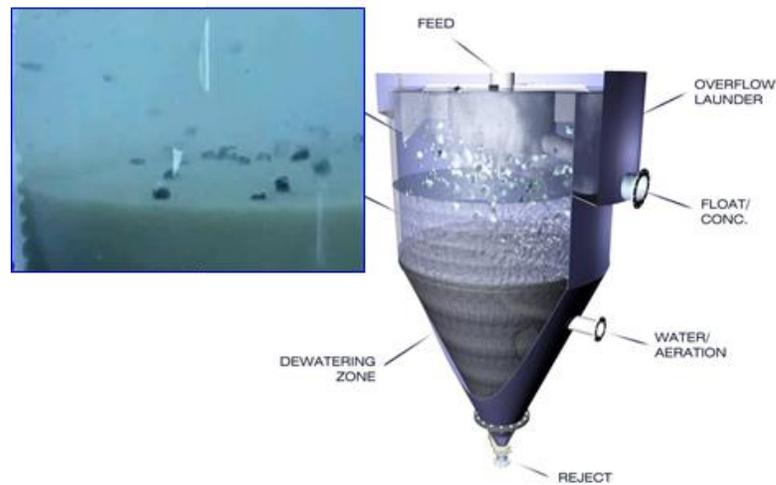
Figure 3 – Schematic illustration of HydroFloat™ separator
