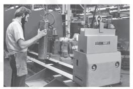
Eriez Bi-Polar Magnets, with a wide range of optional pole-plate configurations, are ideally suited for handling pipe, rounds, bundles, angles and shapes. They can be used in single or multiple-magnet applications.
