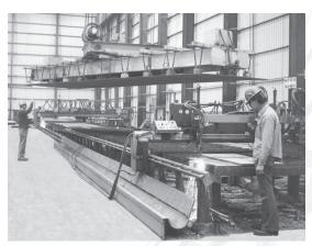
Multiple Selecto Magnets on a lift beam efficiently handle large steel sheets. In this installation, plates up to  $10' \times 50' \times 4''$  (3 m x 15 m x 102 mm) are sorted and transported. The operator has precise remote control of every magnet so those not in use can be turned off, and single sheets can be placed when desired from multiple-sheet lifts.
