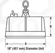
The 18" diameter unit is furnished with a single-chain suspension assembly and single-lead two-conductor powercord.
