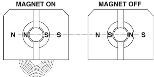
Rotatable element is turned 180° from OFF to ON, or vice versa, to energize or de-energize the magnet.
