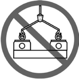
No hooking of two lifting magnets without the use of a properly designed spreader beam.
