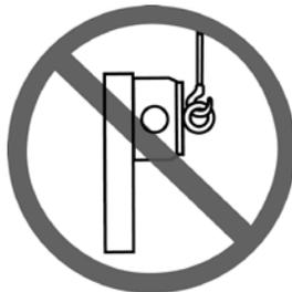
Avoid placing the magnet in shear.
