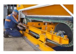
Erie, PA— The latest generation of the <u>Eriez® RevX-E® product line</u> combines the same high performance separation of previous models with a variety of maintenance-friendly enhancements, including an innovative cantilever frame design which enables 10 minute belt changes. The company will present the <u>RevX-E Eddy Current Separator (ECS) with Quick Change belt system</u> in April at both ISRI 2018 and Waste Expo 2018 in Las Vegas, Nevada.
