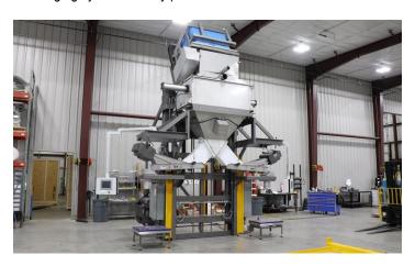
As a global pandemic raged, <u>Material Transfer</u> was called upon to engineer a solution to maintain ice pellet size consistency, meter ice evenly to protect each vaccine, and monitor ice discharged during packaging, all while automating the process. The integrated process includes a crusher, scale system, and customized feeder and controls required to report diagnostics to the vaccine manufacturer.
