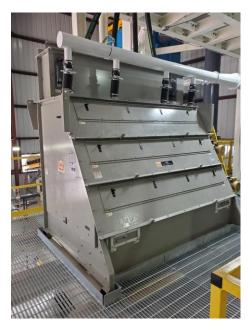
Eriez Rare Earth Roll Magnetic Separators provide maximum efficiency in the separation of weak magnetic particles for product purification applications. Eriez applied sophisticated finite element analysis in magnetic circuit design to produce an energy-free separator capable of generating the exceptionally high field-strengths needed to remove unwanted fine iron contaminants.
