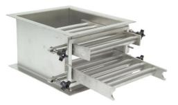
Grates in Housing—Function: Remove ferrous contamination from free-flowing products as it cascades through multiple grate rows within a custom manufactured housing.
